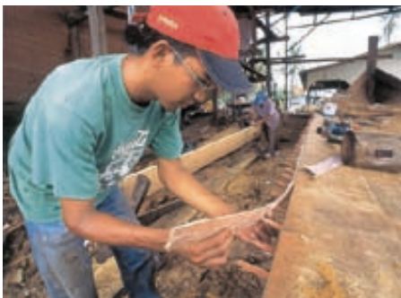
Applying the caulking bark
